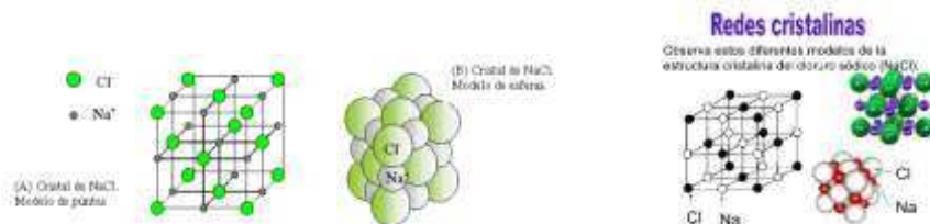
Figura 3.1. Red molecular \text{NaCl}_{(s)}
